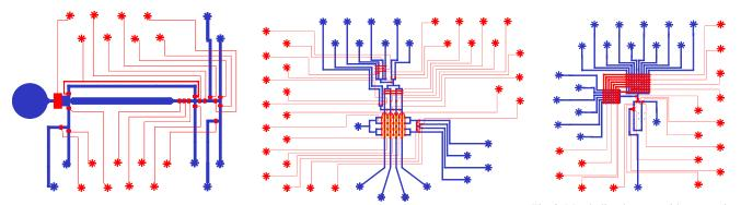
Fig. 6. Cell culture chip with automatic routing. Fig. 7. Waveform generator with automatic routing. Fig. 8. Metabolite detector with automatic routing.
